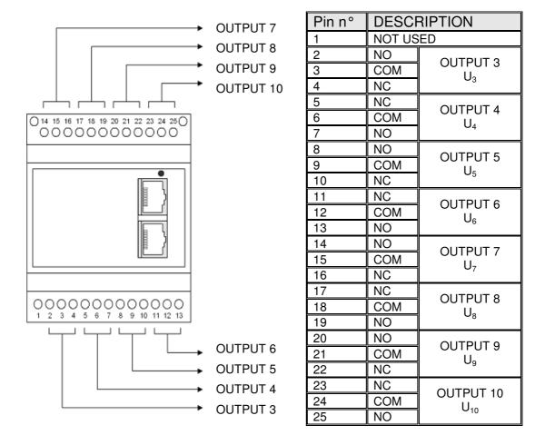
The first time the SMSB26 device is started, all the relay outputs of the SMSB26 device and the output expansions have the contacts set to NC and COM (relay coils not energized).
